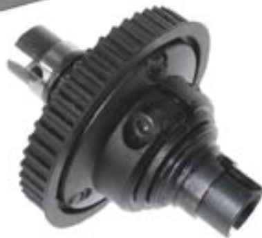
Ball differential using an innovative clamping collar to allow quick and easy adjustment. (Front ball diff optional)
